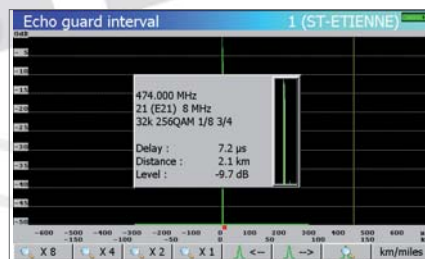
Echo guard interval : Display of echoes, pre-echoes, guard interval with zoom capability.
