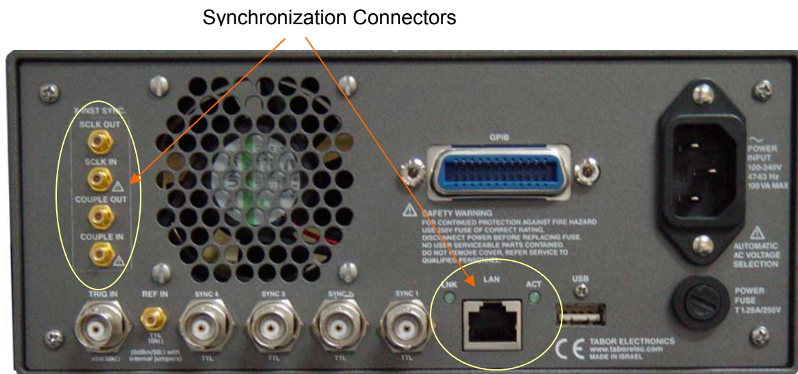
Figure 3-40, Connecting the 2074 Synchronization Cables
