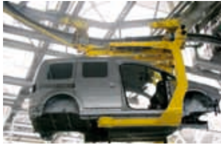
Telpher line positioning in the automobile industry
