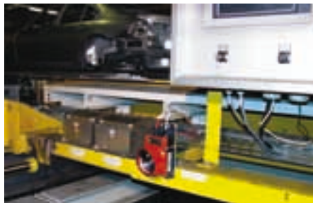
Data transmission to transverse side-tracking skate in the automobile industry
