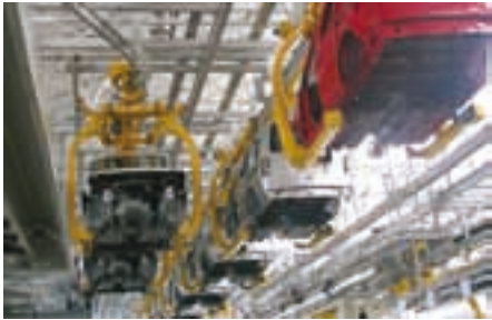
Telpher line positioning in the automobile industry
