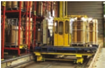
Positioning of transverse side-tracking skates
