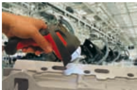
Part tracking for directly marked parts
