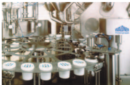
Filling of food containers
