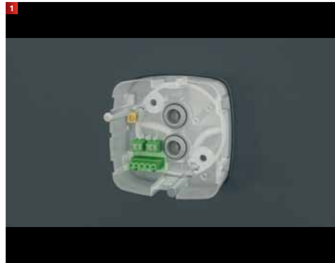
1 Mark-out and drill holes.
