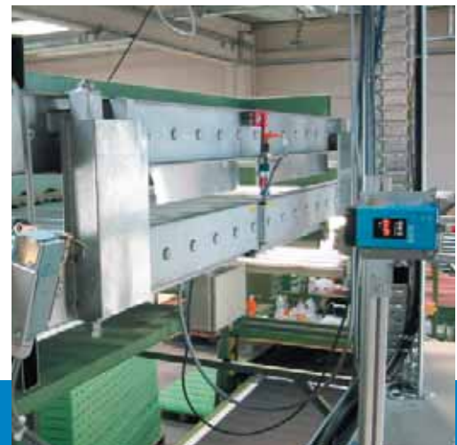
DT500 measuring the position of a foam pad for precise assembly.
