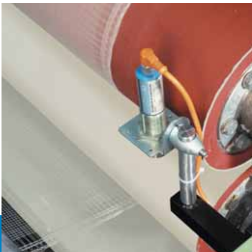
UM18/30 Ultrasonic Sensor measuring clear perforated web.
