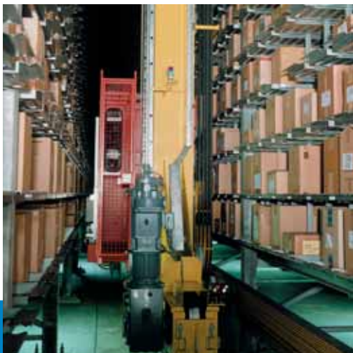
DME, DS60, ISD and other photoelectric sensors in an AS/RS application.
