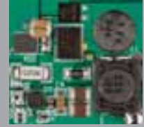
LT3755: SEPIC Demo Circuit. Actual Size, Complete Solution
