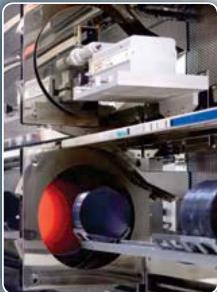
Wafers are brought to very high temperatures in this Thermco furnace to diffuse various N+ or P+ dopants into the areas of the wafer masked off during the masking process.
