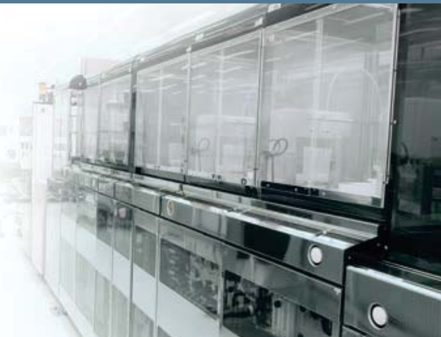
The ASML 5x Stepper aligns the mask to the wafer after the photoresist is spun on.
