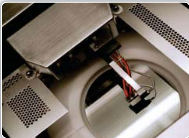
The DNS spin track is an integrated part of the ASML 5x stepper. The spin track applies photoresist to the wafer prior to mask alignment.
