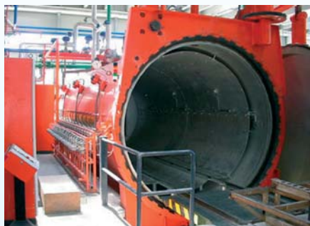
Pressure and vacuum autoclave heating for controlled laminating and curing of technical products for a wide variety of industries.
