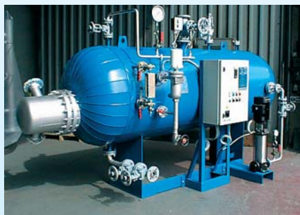
Compact Thermal Fluid heated steam generator. Unfired and inherently safe rapid response for processes where live steam is absolutely necessary, eg humidity control and for existing users not easily converted to thermal fluid heating. Steam at up to 90 bar if required.
