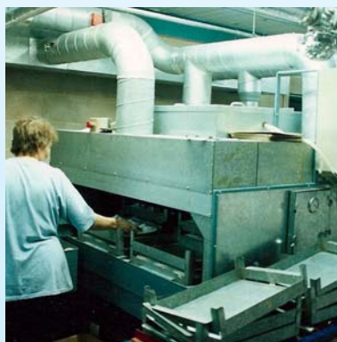
Volume batch production drying for powder and polish manufacture.
