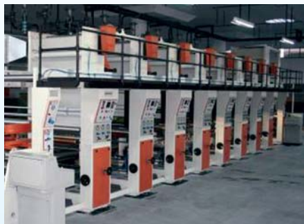
Multi station printing, coating and laminating process. Drier and roll heating applications with cooling if required.
