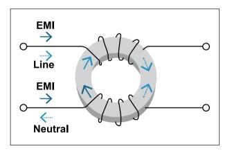
Compatibility (EMC) regulations are more stringent. High frequency (up to 300 MHz) noise can be suppressed with 4S2 cores.
