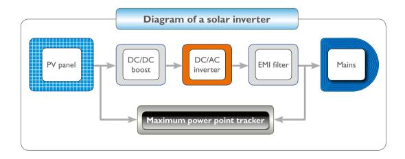
There are several ferrite functions within the inverter: power conversion, EMI filtering and current sensing. The inverter can be split in 4 units:
