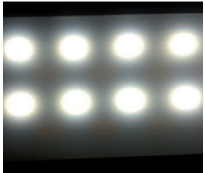
Infineon solution with XMC1000. Flickering (40–50kHz) is neither visible nor detectable by HD cameras.
