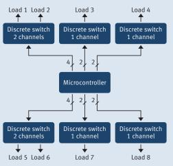
With Discrete Solution: 16 GPIO 8 Channels Output, 8 Diagnostic enable
