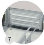
7 Optional 3-slot PCI riser card for 32 bit/64 bit
