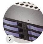
2 Hot-swap HDD module for SATA Interface x 6
