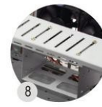
8 Optional PCI hold-down clamp to avoid vibration of add-on card
