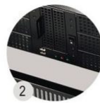
2 LED Indicators- Power, HDD, LAN
