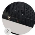
2 LED Indicators- Power, HDD, LAN
