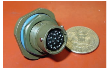
MIL-DTL-38999 Compliant Water Sealed Connector
