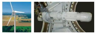
Pitch control functionally independent of line voltage
