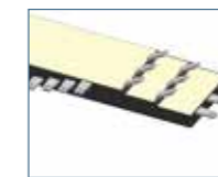
FASTON TABS EXTENDING BEYOND THE BUS BAR OR WITHIN
