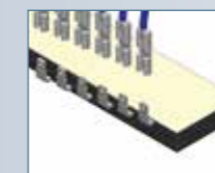
FASTON TABS ALONG THE EDGE WITH FORMS FOR EASY ACCESS
