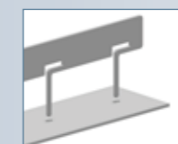
SOLDER PIN CONNECTION WITH THERMAL RELIEF
