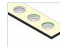
THREE-LAYER BUS BAR UTILIZING EMBOSSED "DIMPLES" FOR COPLANAR INTERCONNECTION
