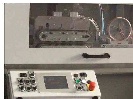
Fig. 4 Control desk with touchpanel and controlled positioning servo drive
