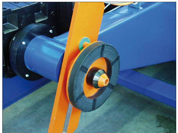
Fig. 10 Frictionally engaged drum driver
