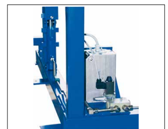
Fig. 4 Hydraulic unit with flow control valve
