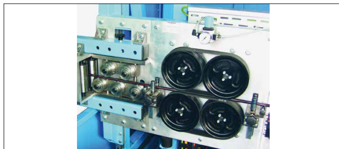
Fig. 2 MESSBOI BELT installed in a machine with roller cages and straightening element
