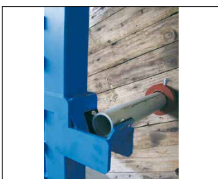
Fig. 3 Drum axle with cone in the device
