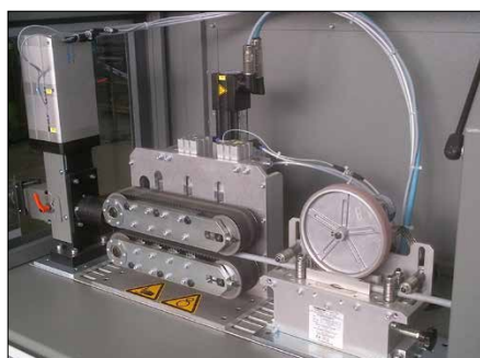
Fig. 2 Installation with a calibratable length measuring device, belt feed and pneumatic cable cutter
