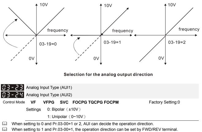
When setting to 1 and Pr.03-00=2, the operation direction can be set by setting 39 of Pr.02-01 to Pr.02-08.
