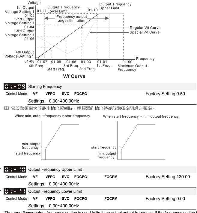
The upper/lower output frequency setting is used to limit the actual output frequency. If the frequency setting is lower than the start-up frequency, it will run with zero speed. If the frequency setting is higher than the upper limit, it will runs with the upper limit frequency. If output frequency lower limit > output frequency upper limit, this function is invalid.
