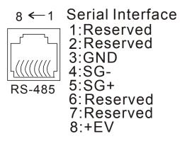
When USB01 needs to use RS-485 port, set the communication speed as 19.2kbits/s and protocol as 8, N,2 for RTU on the computer terminal.
