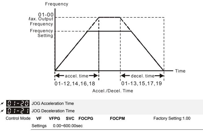
Both external terminal JOG and key "JOG" on the keypad can be used. When the jog command is ON, the AC m motor drive will accelerate from 0Hz (Pr01-07) to jog frequency (Pr.01-22). When the jog command is OFF, the AC motor drive will decelerate from Jog Frequency to zero. The used Accel./Decel. time is set by the Jog Accel./Decel. time (Pr.01-20, Pr.01-21).
