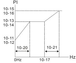
When using multi-function input terminals to switch ASR1/ASR2, the diagram will be shown as follows.
