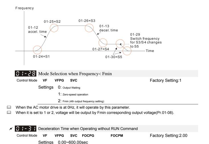
The AC motor drive will stop by the setting of this parameter when canceling RUN command. Refer to the figure in Pr.01-29 for details.
