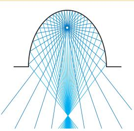
A high efficiency elliptical reflector focuses the bulb's UV energy into a narrow zone. The small diameter bulb also creates a higher peak irradiance at the focal point. End reflectors further enhance the collection of energy to the work surface. Infrared energy, usually harmful to heat sensitive substrates, is reduced by the electrodeless bulb because the small diameter bulb has a lower surface area.
