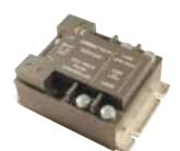
This relay has an analog input isolated from the mains to proportionnally vary the cyclic operating ratio of a load (t/T). Control and mains are synchronous and output only has full periods. Models with LED and RC and VDR network protection.
