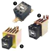
Single phase ready-to-use contactor integrating heatsink, DIN-rail mounting, IP20 terminal protection, LED, VDR, cage terminals... these products are defined with temperature rises of 50°C and permanent 8-hour operation (operating cycles = 100%) in compliance with the European standards
