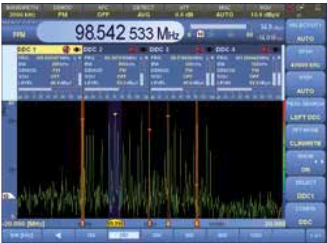
In addition to the main demodulation path (blue), another four signals (red) can be demodulated independently of each other.
