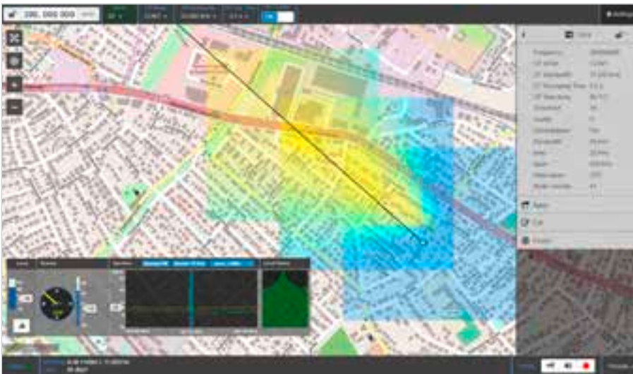
R&S®MobileLocator control software on a laptop or tablet. Display of the current position with vehicle heading, DF spectrum and level versus time, together with the heat map for interference hunting.
