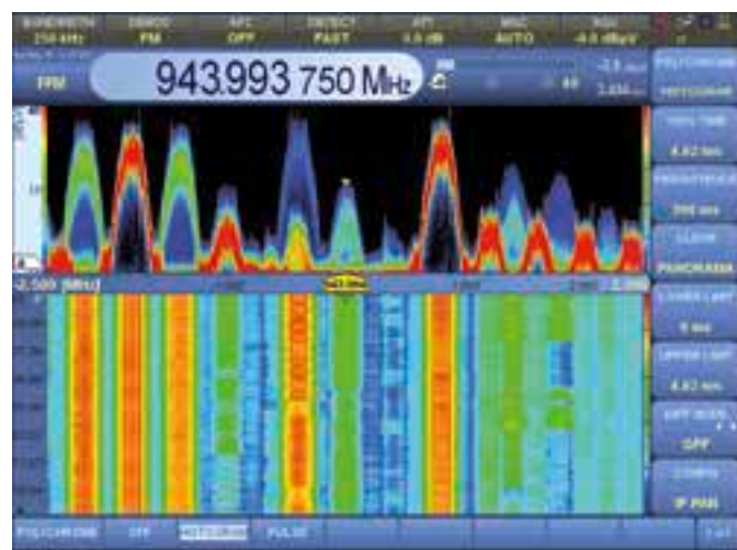
GSM downlink: The histogram mode reveals co-channel occupancy and the different number of occupied timeslots per channel.
