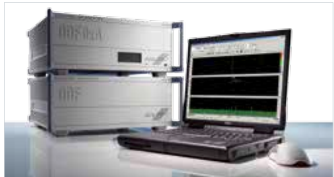
Fig. 16: Typical configuration of a DSP-based direction finder
