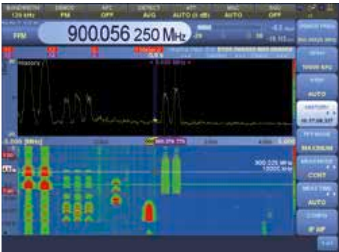
Waterfall display with history and marker functions.
