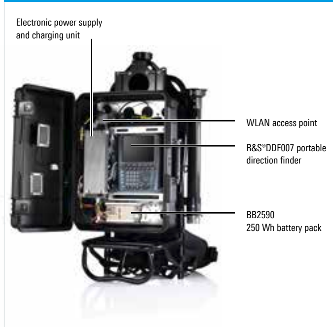
Backpack integration with the R&S®DDF007, battery pack with 250 Wh, electronic power supply and charging unit and WLAN access point. For extended operation time, a solar panel can be used with system.
