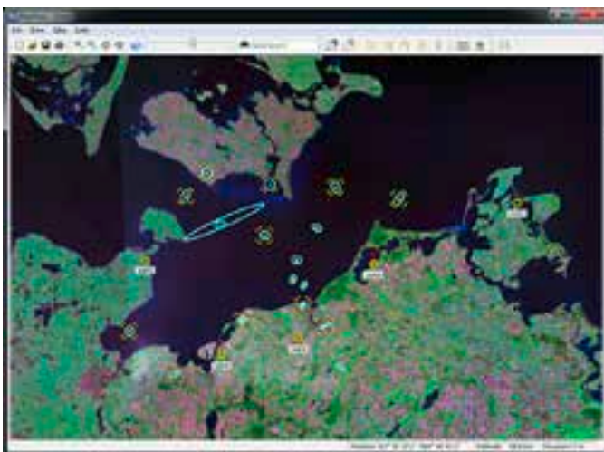
Map display on an operator's monitor. Different symbols are used to designate different transmitter categories.
