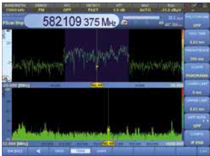
IF spectrum, with selected demodulation bandwidth highlighted in blue. Lower part: panorama scan.
