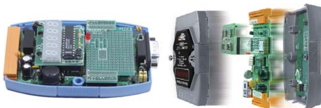
Plug an X-Board into a palm-size PAC
