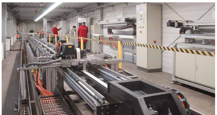
Drag chain test system
