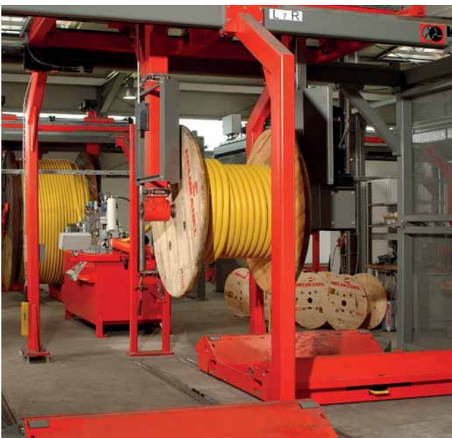
Heavy-load, cable-cutting facility
