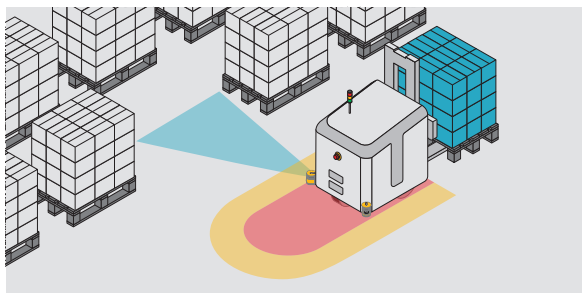
Direct navigation of AGV thanks to monitoring of the environment.
