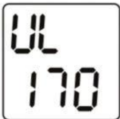
170V under voltage protection
