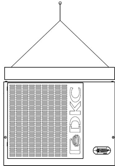
The coolers may be mounted inside or outside the enclosure. The cooler must always be installed horizontally with the maximum standoff from the upright position equal to 2°.
