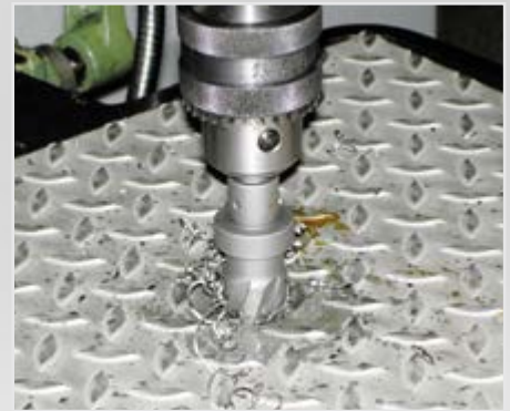
Drilling structured sheet metals
