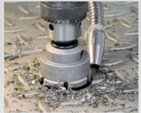
Drilling in checker sheet
