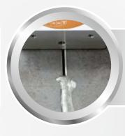
Magnets allow welding at a distance of just 15 mm (9/16") from the magnet's external side
