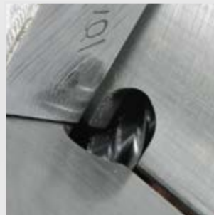
Precise deburring by rolling milling
