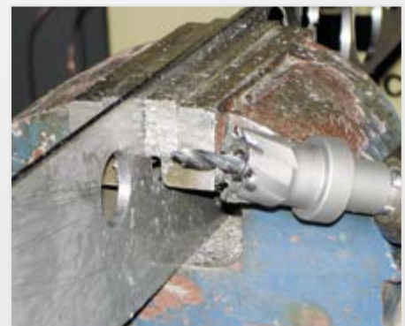
Free-hand drilling up to Ø 30 mm
