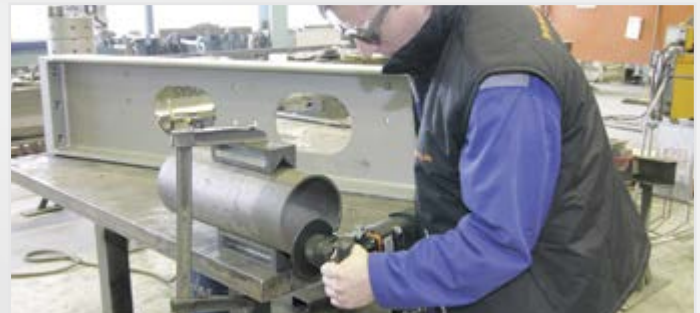
Start holes from \varnothing 20 mm.
