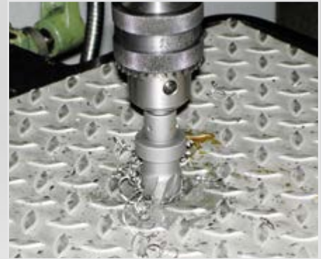
Drilling structured sheet metals
