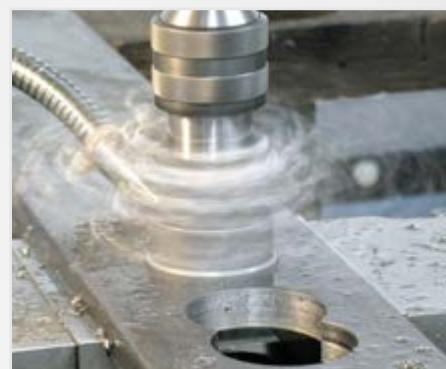
Drilling in flat steel
