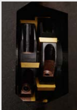
2 milling disks together with 6 inserts each
