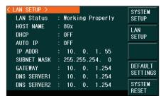
Integrate your LCR meter into an automated test system and control it from a PC using SCPI commands via the RS232, USB, LAN, or GPIB interface.
