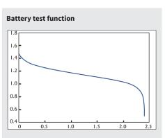
The built-in battery test function uses CC mode to calculate the battery capacity using a fixed current load discharge. Users can specify cut-off voltage level, capacity level and time stop conditions.
