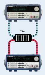
Couple the 8500B load with power supplies such as the 9115 or 9200 series to perform charge/discharge tests on batteries.
