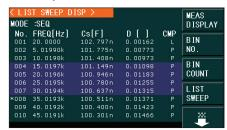
Use the built-in sweep function to conveniently display, analyze and store primary and secondary parameters of a component at up to 201 frequencies.
