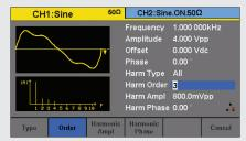
Generate up to 10 harmonics with independent amplitude and phase settings.
