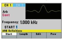
From the front panel, waveforms can be defined from scratch by entering data point-by-point or by loading and modifying predefined waveforms.
