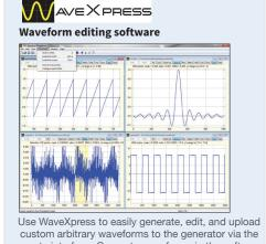
Use WaveXpress to easily generate, edit, and upload custom arbitrary waveforms to the generator via the remote interface. Generate waveforms in the software by importing a text file or define via freehand, point draw, and waveform math functions.
