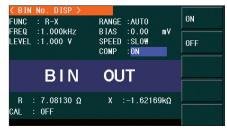
Use the BIN comparator function to sort components in up to 10 bin locations.
