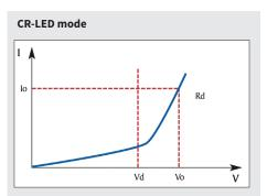
Use the load's unique CR-LED operating mode to test LED drivers. This function allows users to configure the LED's operating resistance and forward voltage to simulate the loading behavior of typical LEDs.
