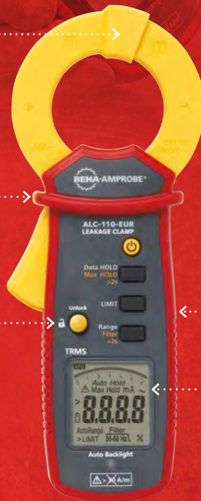
ALC-110-EUR Leakage current clamp meter
