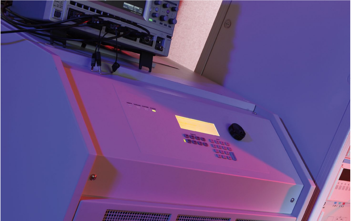
45 kVA Electronic power source (AC+DC) with a power up to 45 kVA. For simulating worldwide power quality situations and failures.
