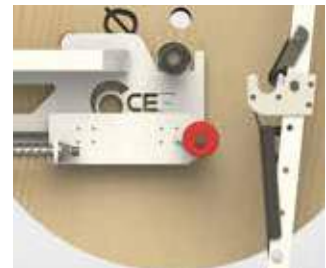
The forklift extension loses contact with the hook and the safety lock closes automatically.
