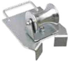
CODE 0281 Zinc-coated steel drum cable layer with rotating support on an angle base to be used on the edges of wells.
