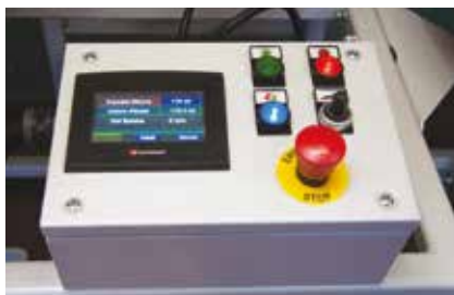
CONTROL PANEL WITH TOUCH SCREEN PLC To set the measure to take and manual handing.
