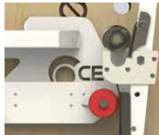
The forklift lifts the drum and the safety hook remains in the open position.
