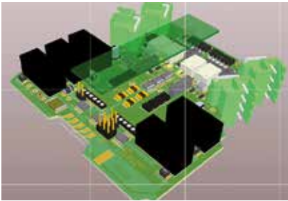
Altium 3D circuit board layout
