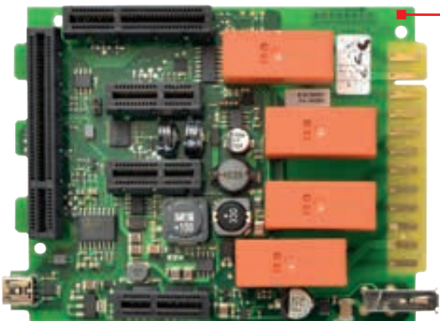
Relay card with 4 changeover contacts
